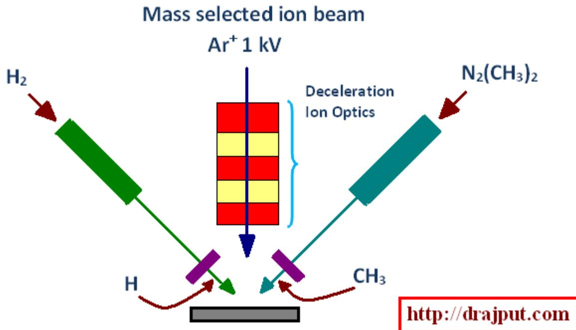
In this experiment, the very first step is the creation of dangling bonds at the film surface. Dangling bonds are created by abstraction of surface-bonded hydrogen by impinging H and CH<sub>3</sub> radicals. Chemisorption of CH<sub>3</sub> radicals at dangling bonds at the C:H film surface results in
