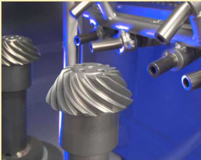
Shot peened gear Metal Improvement Company Paramus, New Jersey
