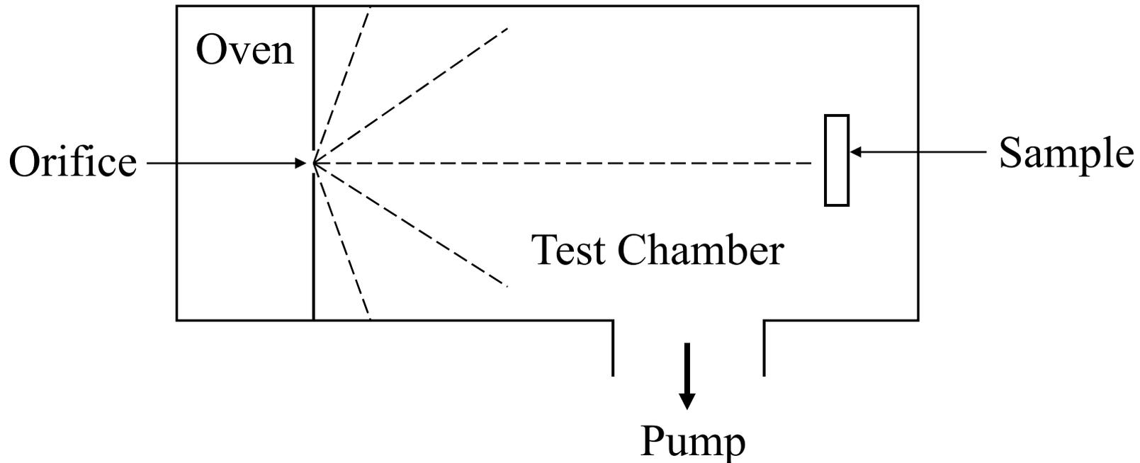
Knudson cell effusion beam system
